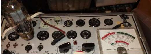
KT66 tests like new Passes gas test too.
